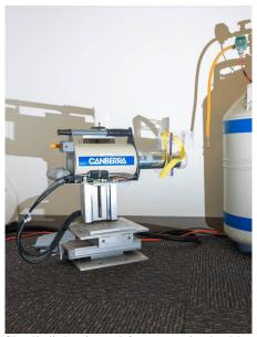
A machine, nicknamed "Charlie," that is used for measuring lead levels in a person's bones at Mount Sinai Hospital in New York.
